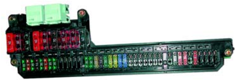
Front Power Distribution Box
